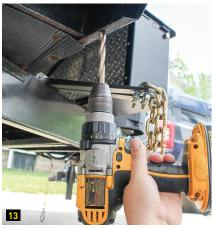
11) The spring bars slide through the bracket and can be locked to the frame using the optional Master Python Adjustable Cable Lock or (12) a long-hasp padlock. How they are inserted into the bracket depends on the spring-bar type. 13) The spring bars can also be locked to the crossmember by drilling a hole in the wing and threading the cable through the hole.
